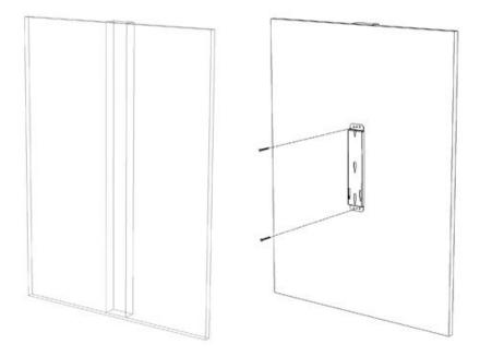
3. Insert the enclosure screws into the enclosure, as shown. Tighten the screws until approximately 2 mm of thread are visible.
